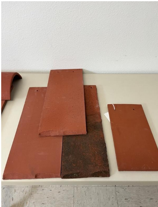
FIGURE 7: EXISTING AND REPLACEMENT TILES DURING PILOT TILE SELECTION FOR 732 LIGGETT
