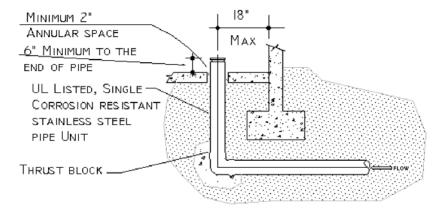
5.10 Piping shall be installed a minimum of 12 (twelve) inches (300 mm) below the bottom of building foundations or footers.
