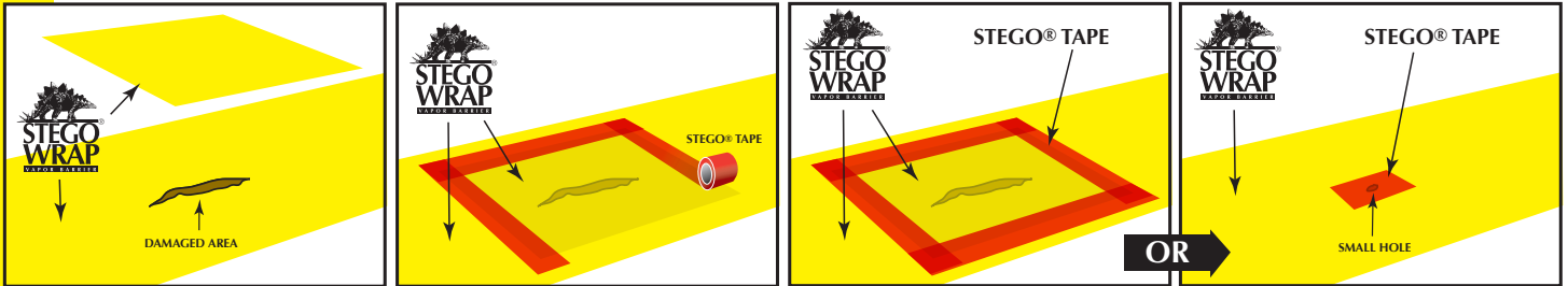
FIGURE 3: SEALING DAMAGED AREAS
